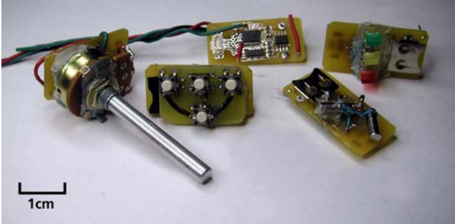
Figure 7. Wireless components: (left to right) analog knob, 4-button array, master uplink transceiver, 2-axis tilt sensor, and 3-LED array.
