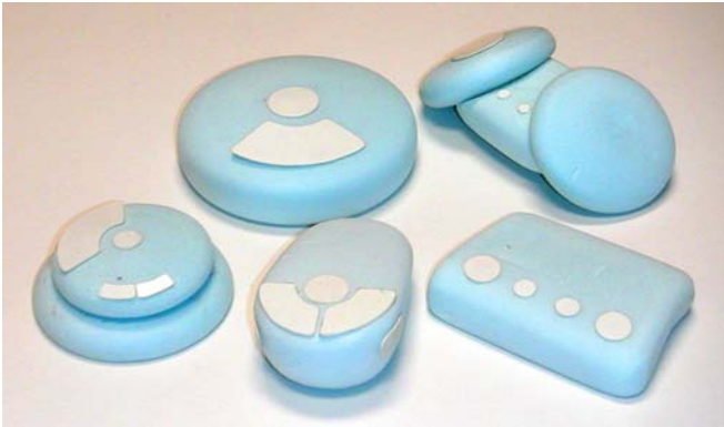
Figure 1. Designers often use blocks of foam material to generate sketches of form.
